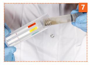
Insert the sample tube into the strip tube.
