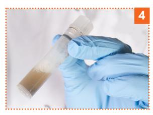
■ Shake the sample tube to homogenize well.
