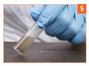
■ Tap the sample tube on a hard surface so that all the liquid is collected at the bottom of the tube.
